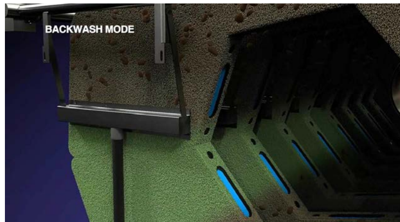
Figure 7: Backwashing and removal of solids.
