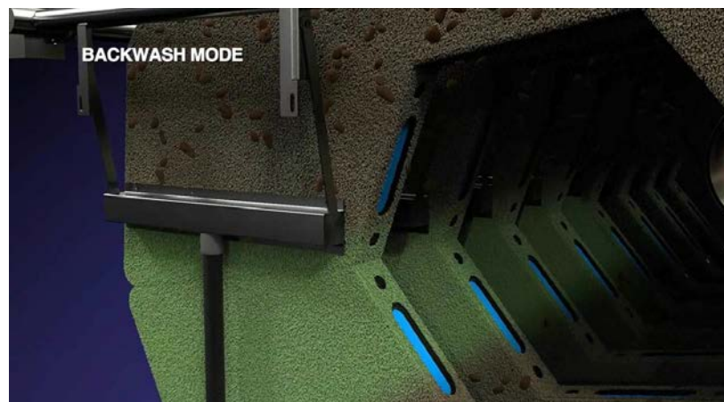
Figure 7: Backwashing and removal of solids.
